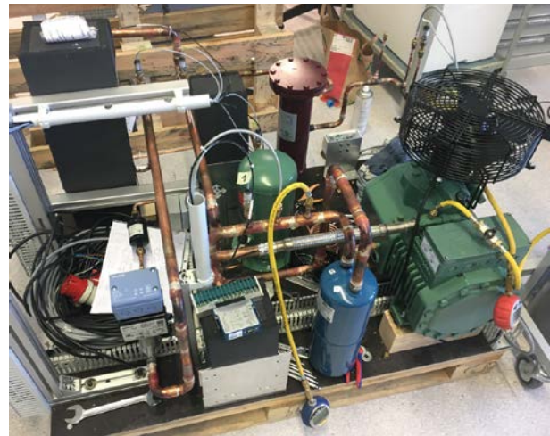
Figure 2: High temperature heat pump demonstrator prototype in construction at NTB Buchs.
