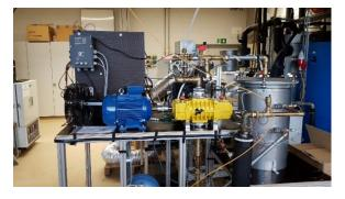
These two experimental systems validated the previous studies, which showed that a high temperature heat pump combined with mechanical vapour recompression is the most beneficial method of generating steam in terms of efficiency and technology readiness level. However, in building the open loop water heat pump, it has been confirmed that there is a lack of steam compressor availability in the actual market.
